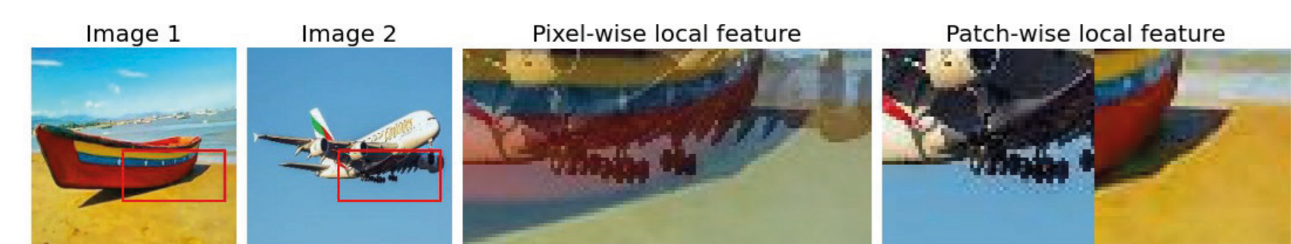
Figure 4. From left to right: two sample images and examples of pixel-wise and patch-wise mixing, respectively. The pixel-wise and patch-wise images present the zoomed region indicated by a red rectangle to show the detailed characteristics of the mixed images. Source: [8].
