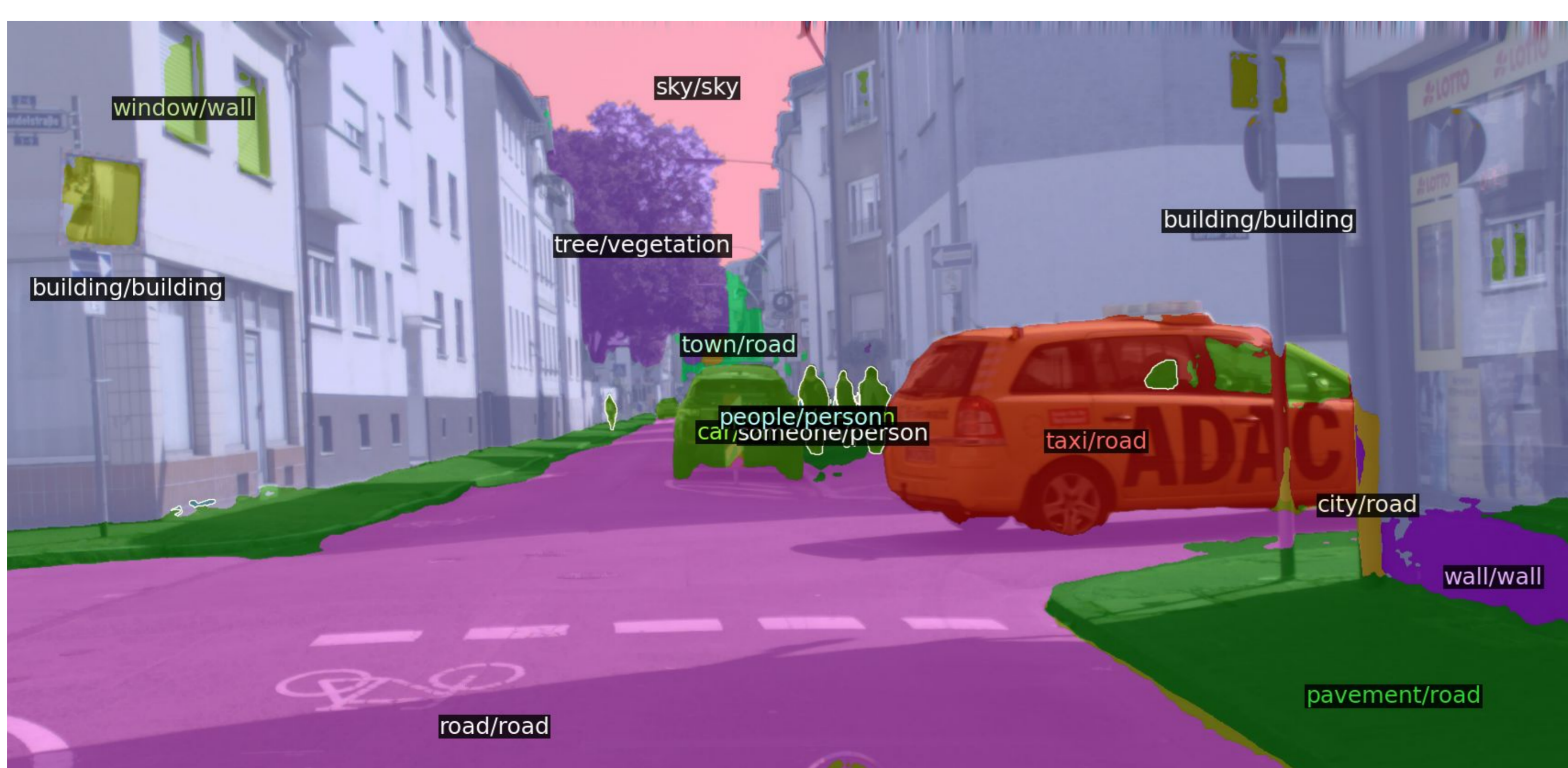
Example output of our method, with generated label on the left and the closest Cityscapes class on the right. The "taxi/road" mapping is a clear mistake
